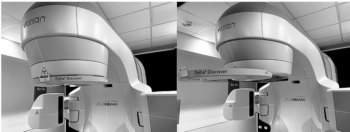
Fig. 1. Delta<sup>4</sup> Discover mounted on a Varian Truebeam Linac.
